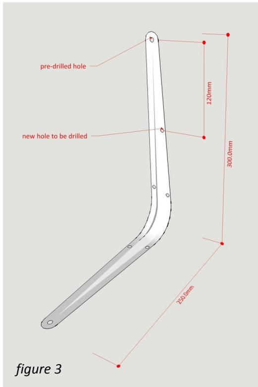
3. Using one bracket line it up with the length of pipe and ensure that it overhangs the end by 150mm. mark the holes needing to be drilled and repeat 3 times around the circumference of the pipe. Drill the holes – [see figure 4]
