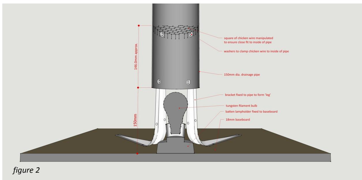
2. Take a bracket and note that the shorter leg (250mm) will be fixed to the baseboard. On the longer leg (300mm) mark and drill a hole the same size as the pre-drilled hole at approx. 120mm down from the pre-drilled one. Repeat this process for the 3 remaining brackets – [see figure 3]
